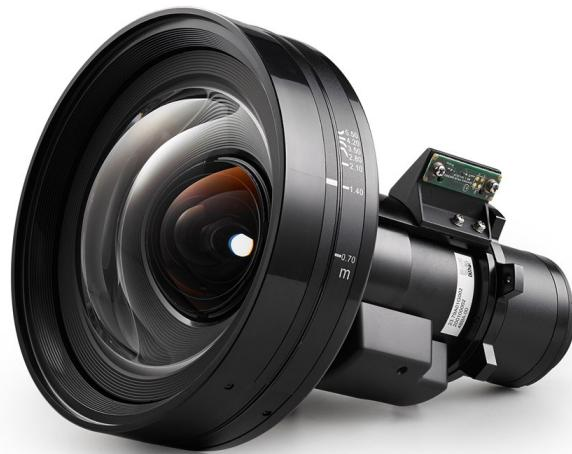
The BX-CTA17 short-throw lens is ideal for immersive installations that require a short distance between the projector and the screen. With a throw ratio of 0.65 ~ 0.75:1, it can easily project images from 50 inches up to 1,000 inches.
